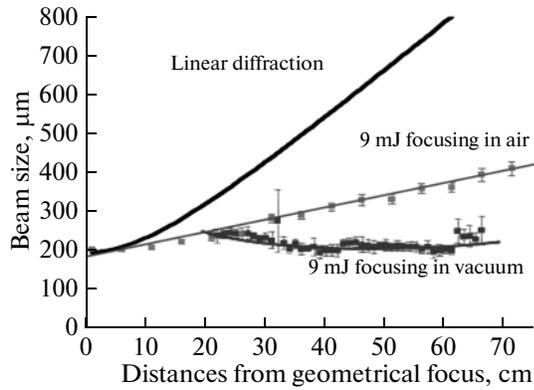
**Fig. 5.** Width of successive profile measurements taken at various distances from the aerodynamic window. At low energy, the profiles follow the linear diffraction theory curve (shown in black).
