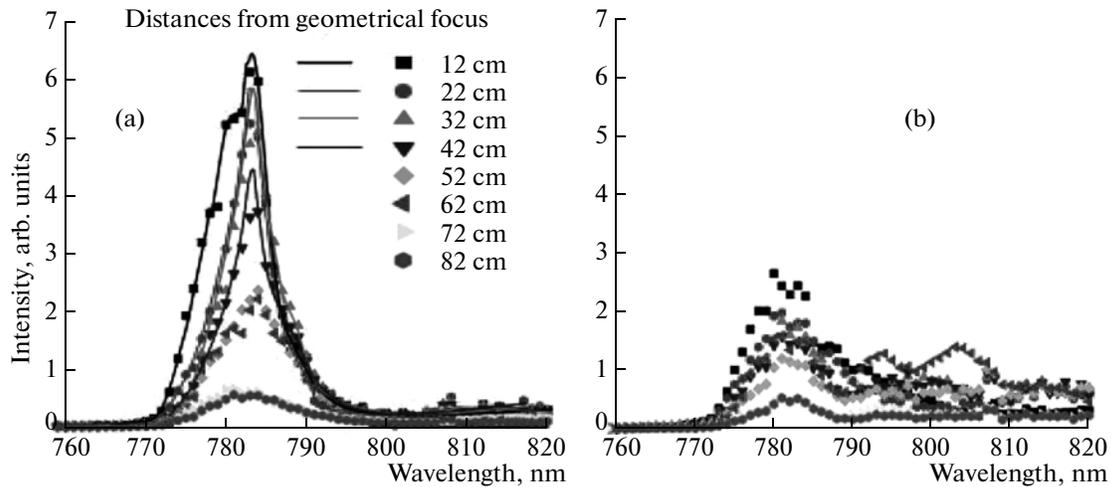
**Fig. 3.** Spectra recorded at various distances from the geometrical focus of the 3 m lens are displayed for the case of (a) focusing in vacuum (aerodynamic window on) and (b) focusing in air (aerodynamic window off).
