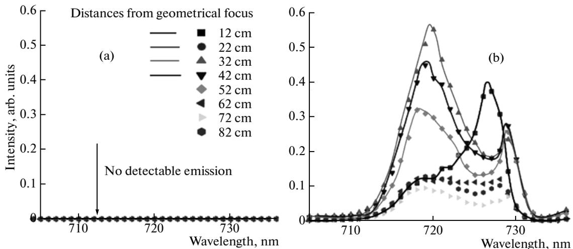
**Fig. 4.** New wavelengths generated in the blue region of the spectrum, recorded at various distances from the geometrical focus of the 3 m lens: (a) focusing in vacuum (aerodynamic window on) and (b) focusing in air (aerodynamic window off).
