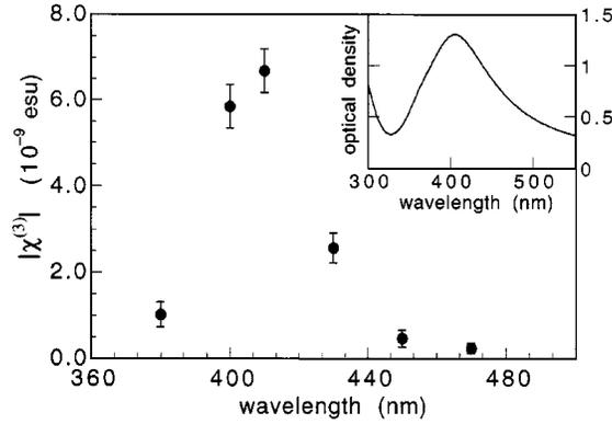
Fig. 3. –  $|\chi^{(3)}|$  dispersion for a layer of Ag nanoclusters embedded on a glass substrate. Optical absorption of the sample is reported on the inset.
