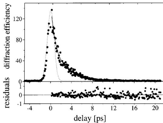
Fig. 4. – Temporal response of the FWM signal (No. 4) measured by delaying one of the pump beams (No. 3). Dashed curve:  $\chi^{(3)}$  autocorrelation of the laser pulse, obtained with the sole substrate. Full line: fit with three exponential decay curves, of 0.9, 3 and 30 ps. The normalized residuals are shown to underline the quality of the fit.
