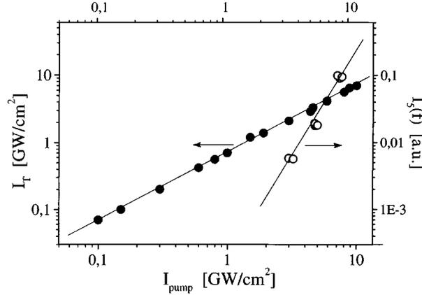
Fig. 2. – Right: example of the cubic dependence of  $I_5$  on the incident pump intensity at 400 nm. The linear fit has slope  $3.15 \pm 0.2$ . Left: transmitted intensity of the glass substrate at 400 nm.
