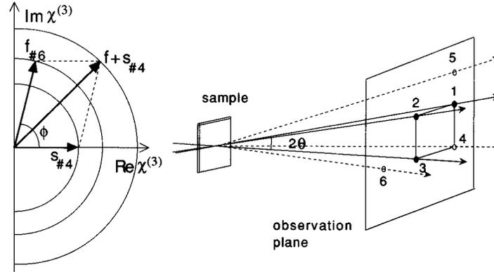
Fig. 1. – Left: diagram in the complex  $\chi^{(3)}$  plane showing the quantities evaluated from measurements. Amplitudes of  $\chi^{(3)}(f)$ : central arc;  $\chi^{(3)}(s)$ : inner arc;  $\chi^{(3)}(f, s)$ : outer arc. Right: scheme of the beam geometry used in the DFWM experiment.
