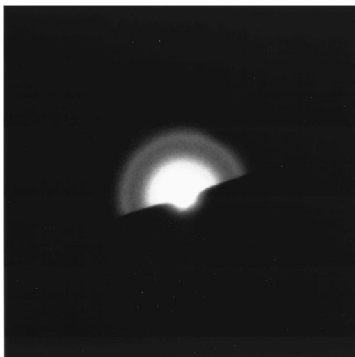
FIG. 2. Selected area diffraction pattern showing crystalline rings from a poled silica sample.
